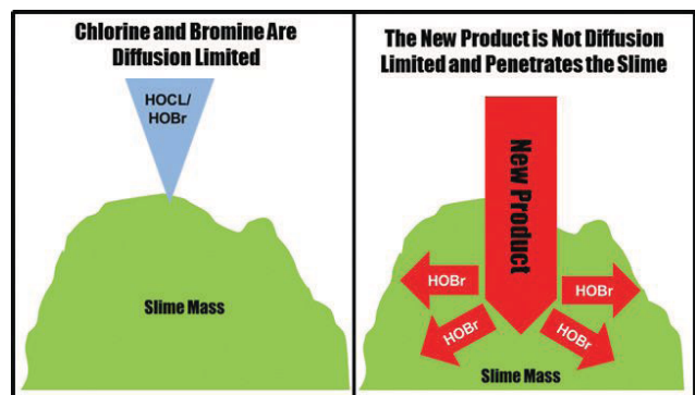
Figure 2. The stabilized, chlorine-based cooling water biocide penetrates into slime and produces bromine in situ to break up slime masses from within.
